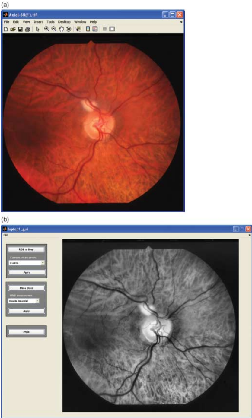
Fig. 6 (a) An unenhanced RGB image showing moderate delineation of the blood vessels. (b) Image in (a) after greyscale conversion and CLAHE enhancement. The retinal vessels are clearly more prominent.
